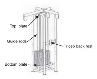
Figure 9. Remove the tricep back rest, the top plate and the guide rods.
